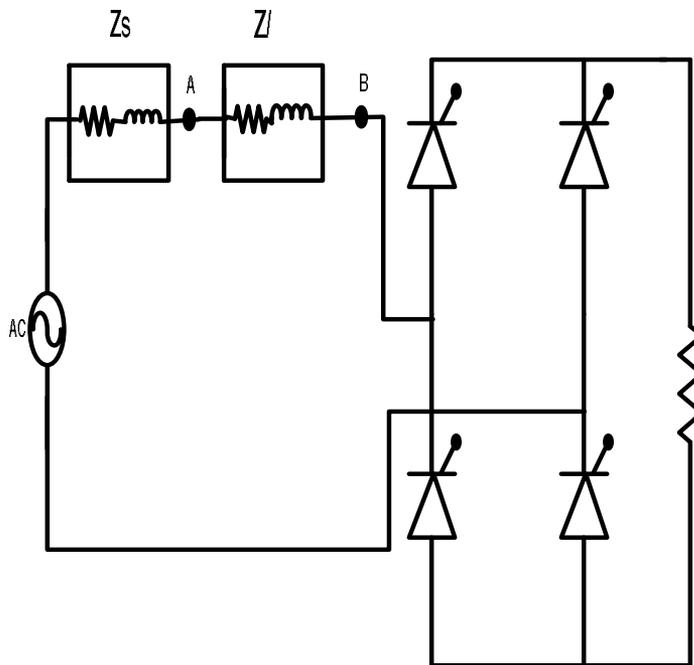
**Figure 2.** Nonlinear load with R load connected to a AC supply
