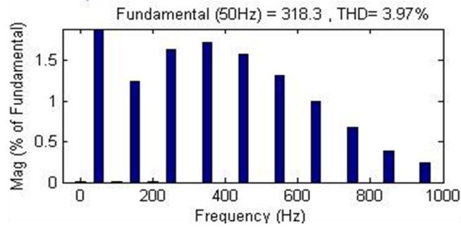
**Figure .7.** Total Harmonic Distortion of Voltage at Node 1 shows 3.97% with  $\alpha=30$  controlled R load
