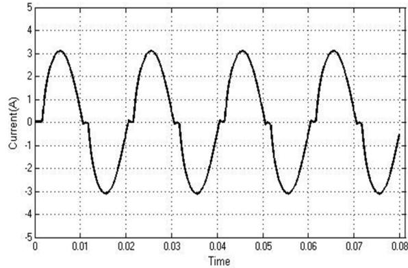
**Figure .10.** Simulated Current wave form at Node 2 with  $\alpha=30$  controlled R load
