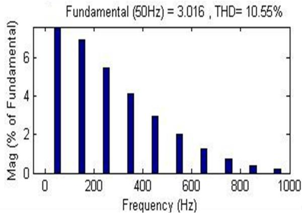
**Figure .8.** Total Harmonic Distortion of Current at Node 1 shows 10.55% with  $\alpha=30$  controlled R load
