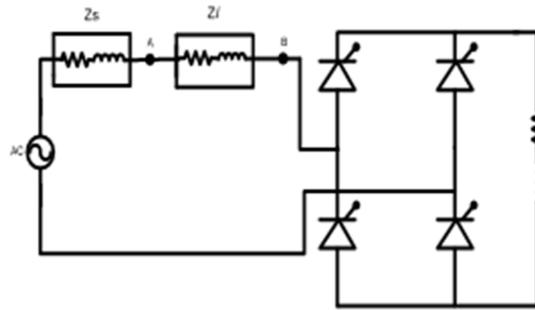
Figure .3. Nonlinear load with RL load connected to a AC supply
