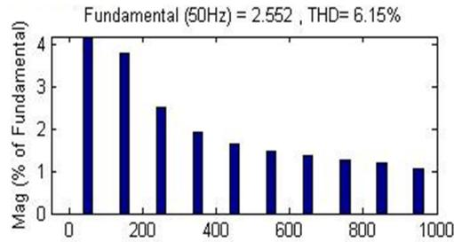
Figure .16. Total Harmonic Distortion of Current at Node 1 shows 6.15% with  $\alpha=30$  controlled RL load
