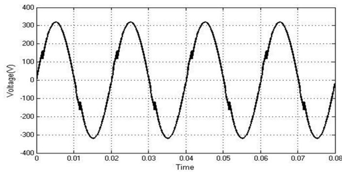
Figure .5. Simulated Voltage wave form at Node 1 with  $\alpha=30$  controlled R load
