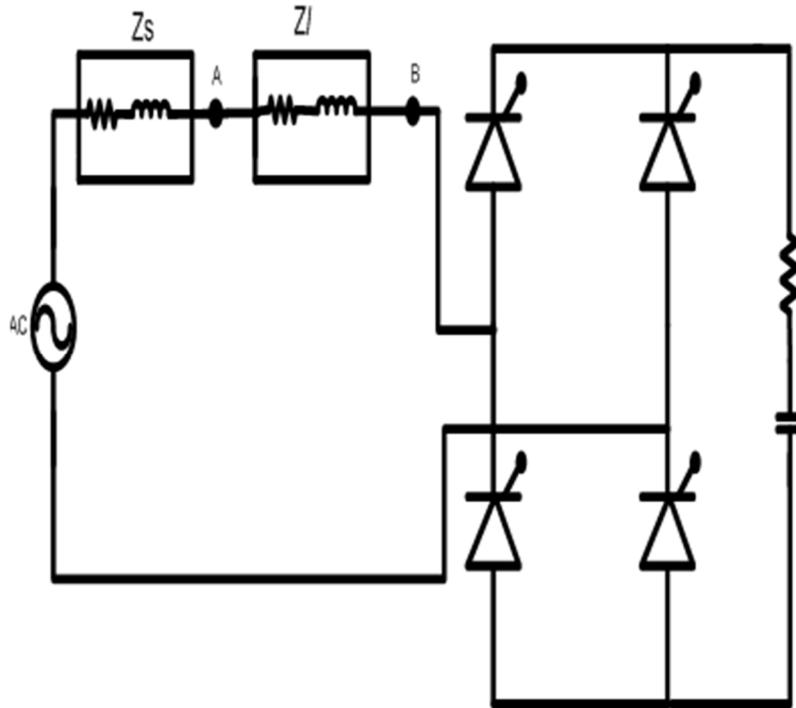
Figure .4. Nonlinear load with RC load connected to a AC supply
