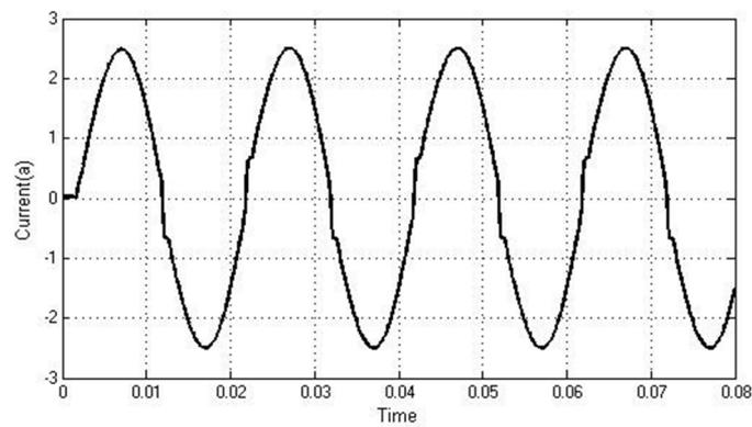
**Figure .14.** Simulated Current wave form at Node 1 with  $\alpha=30$  controlled RL load
