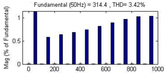
Figure .15. Total Harmonic Distortion of Voltage at Node 1 shows 3.42% with  $\alpha=30$  controlled RL load
