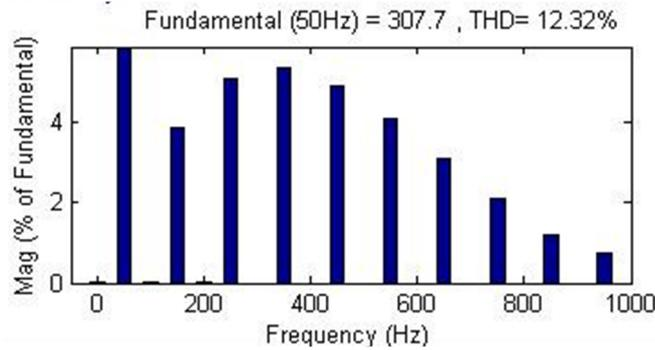
**Figure .11.** Total Harmonic Distortion of Voltage at Node 1 shows 12.32% with  $\alpha=30$  controlled R load
