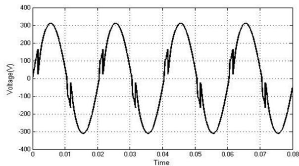
**Figure .9.** Simulated Voltage wave form at Node 2 with  $\alpha=30$  controlled R load
