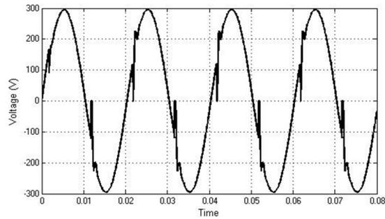
Figure .17 Simulated Voltage wave form at Node 2 with  $\alpha=30$  controlled RL load
