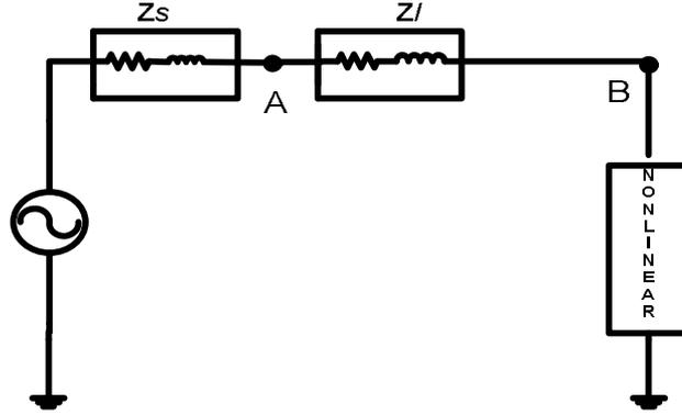
Figure 1. Simple network with a nonlinear load connected to a sinusoidal supply
