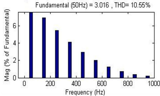
**Figure .12.** Total Harmonic Distortion of Current at Node 2 shows 10.55% with  $\alpha=30$  controlled R load
