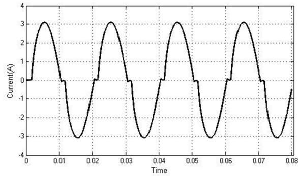
**Figure .6.** Simulated Current wave form at Node 1 with  $\alpha=30$  controlled R load
