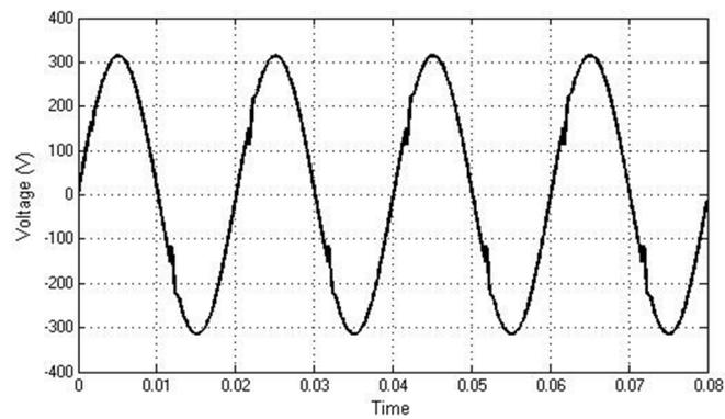
**Figure .13.** Simulated Voltage wave form at Node 1 with  $\alpha=30$  controlled RL load
