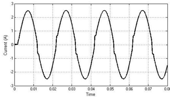
Figure .18 Simulated Current wave form at Node 2 with  $\alpha=30$  controlled RL load
